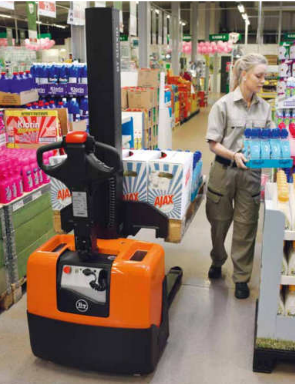
The HWE100 is the simplest model in the BT Staxio W-series – a compact truck that provides safe, easy horizontal pallet movement and stacking in low-intensity applications. The HWE100's low weight, compact size and 1000 kg load capacity make it ideal in a wide range of applications.
