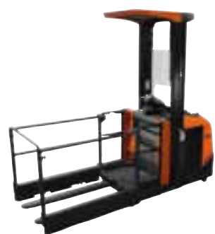
OME100N with auxiliary lift and OME100NW walk-through version • Chassis width 810 mm • Maximum capacity 1000 kg • Picking heights to 3.4 m
