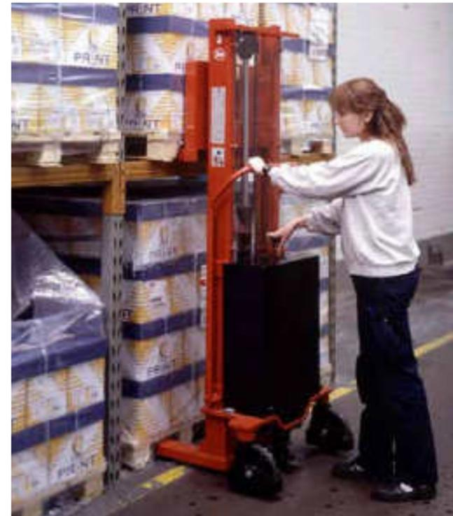
Load capacity: 0.8 t @ 600 mm load centre
