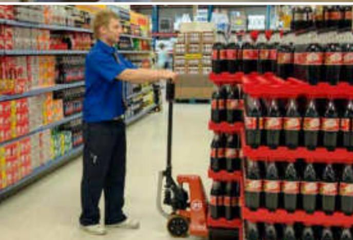
For nearly effortless movement of goods, the BT Pro Lifter (LHT100) has an electric motor built into the main wheel. This means that loads of up to one tonne can be moved at the touch of a button.
